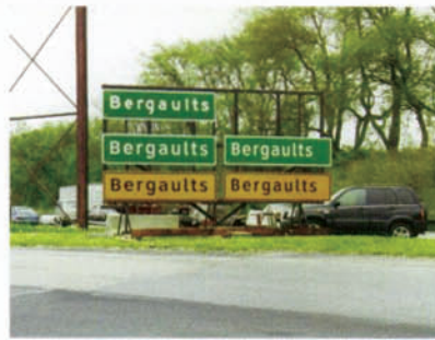
top Clearview on Pennsylvania's Route 171 above Five different versions of the font in a test rack
